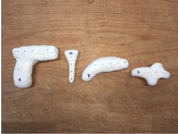
Fig. 4: Clay models of the handle prototypes. From left to right: pistol, pen, nunchuck and hybrid.
