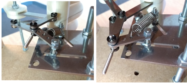
(a) Orientation of the system when the hand is opened. (b) Orientation of the system when the hand is closed.
