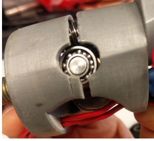
Fig. 4: Due to faulty orientation of printing and the forces exerted on the housing, an earlier design broke. Here, the fault line can be seen [11].
