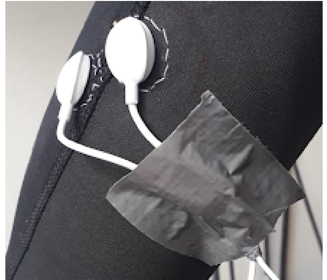
Fig. 3. EMG sensor taped to the shirt
