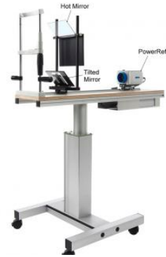
Figure 1: Set-up of the experiment with the PowerRef III
