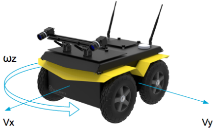
Fig. 1. Clearpath Robotics' Jackal with a representation of v_x , v_y and \omega_z .
