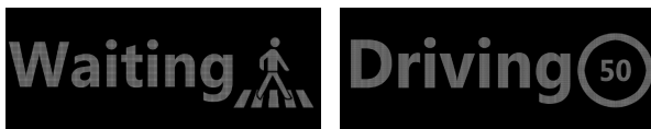
Fig. 3.2. The eHMI message displayed when the car is going to stop (left) or continue driving (right)
