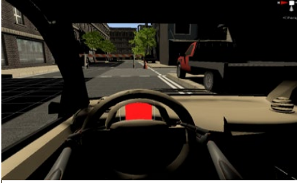
Fig. 4. Collision warning in Smart in the experiments' VR world
