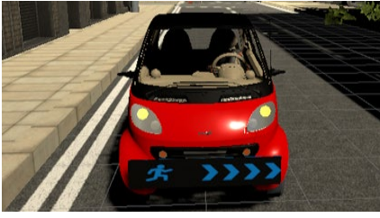
Fig. 3. Driveable Smart with eHMI to the right in the experiments' VR world
