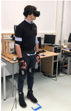
Fig. 2. A pedestrian participant wearing the Xsens motion suit and Oculus Rift in the experiment surrounding.
