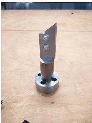
Fig. 8. Utility knife end effector
