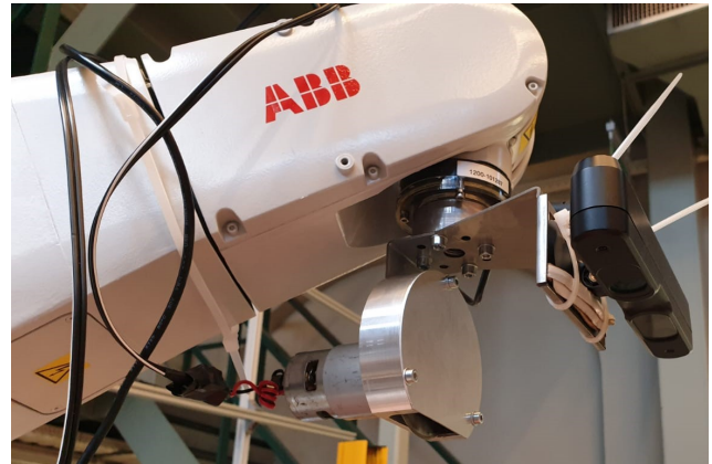
Fig. 10. End effector (circular blade + 3D scanner) mounted at the end of the ABB IRB1200 robotic arm
