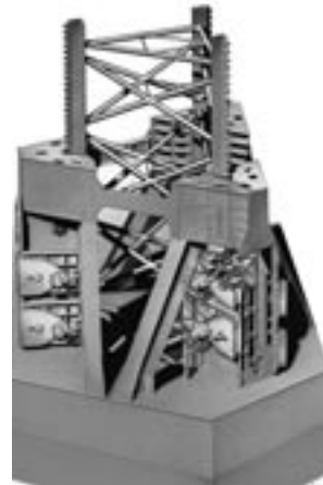
Hydraulic rack and pinion elevating system, IHC Gusto Engineering
