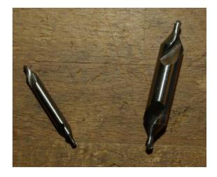
Centre drills depend on the size of the final hole to be drilled. The dimensions of the thin drill section and the shank dimensions are indicated on the centre drills.
