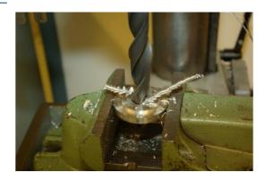
If you have to exert too much pressure on the drill while drilling, this will usually mean that the drill is either blunt or unsuitable for the material you are drilling in. There is then a good chance
