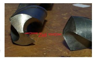
A common mistake is to perform this pre-drilling in steps with a drill that is only a couple of millimetres larger, until we reach the right size. It is better not to do this because a drill that is only a couple of millimetres larger will tend to grab in the hole that was previously drilled.
