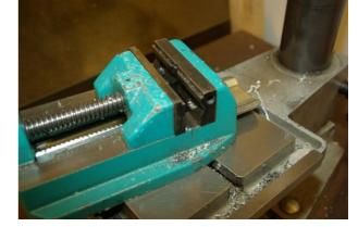
drill bits. Make sure that the underside of the material is free of the machine vice so that the bit does not damage the machine vice guides when it emerges from the workpiece.
