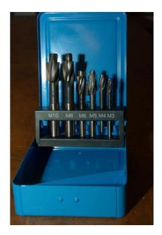
countersink holes for countersunk head screws. In that case, the cutting part is ground at an angle of  $45^{\circ}$ .
