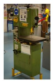
In the case of a vertical band saw, the saw runs over two wheels that are mounted vertically above each other.
