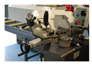
With a horizontal band saw, the two guide wheels are set up horizontally at an angle, with the band saw making a horizontal sawing motion.
