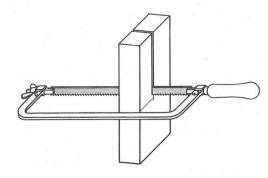
To saw off parts that are higher than the saw-frame, most saw-frames allow the saw to be clamped at 90°. However, it will then be necessary to remove and reclamp the saw.
