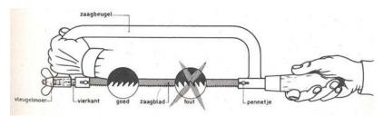
Saws are placed in the frame with the teeth facing forwards and clamped using the tightening screw or handle (depending on the make of the saw frame) so that the saw blade is taut.
