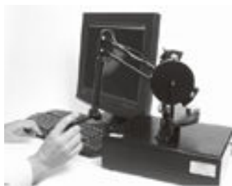
Fig.1 PHANToM haptic device
