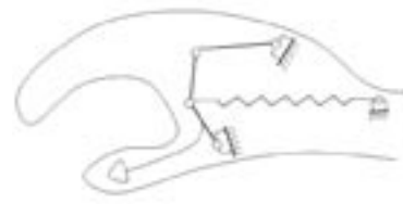
Fig.3 Four bar linkage for compensation mechanism Fig.4 Four bar linkage
