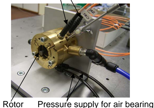
Optical probe for measuring vibration amplitude
