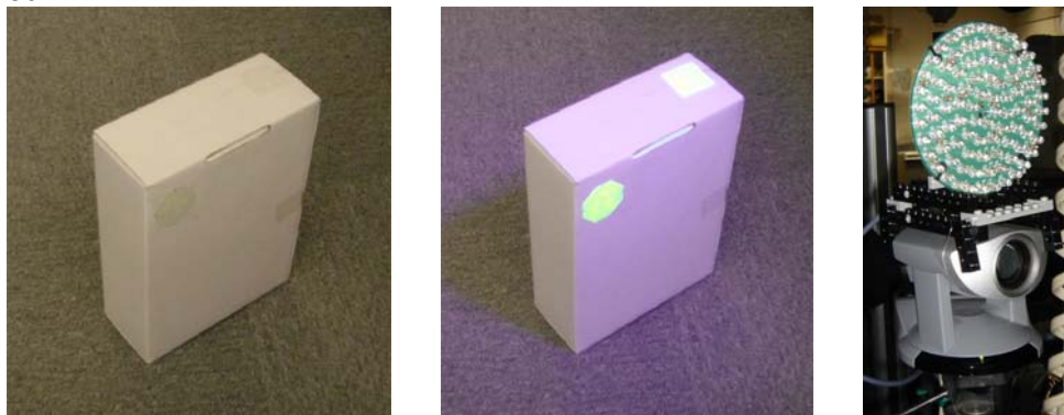
Fig. 6 Fluorescing PenTag without and with UV-light & UV-source
