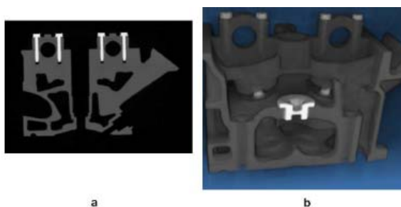
Fig. 2: Engine head scanned by Toyota: (a) Cross section obtained by scanning, (b) Volume rendered reconstruction from CT data
