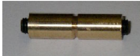
Fig 6: Pictures of the work piece holder with rubber rings
