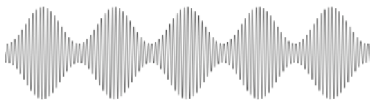
Figure 1. Schematic representation of an amplitude modulated ultrasonic vibration, with a sinusoid signal wave.
