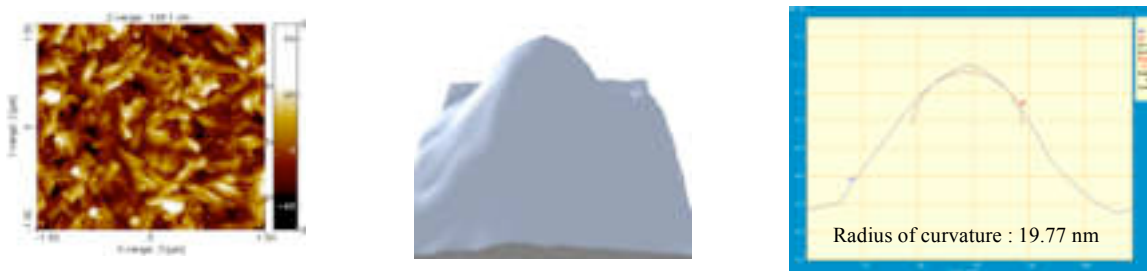
(a) TipCheck image (b) Estimated tip shape (c) Estimated tip shape profile
