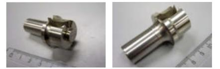
I measured roughness of the surface with Form Talysurf Series 120L (Taylor-Hobson). I did not do finish machining because of lack of time. Therefore roughness is not good enough for rotor. The smoothest part is outside of the blade. The reason why this part gets the smoothest surface is this side was machiened pertically. The roughest side is machined not pertically. But even the smoothest surface is not good enough for a micro turbine rotor.
