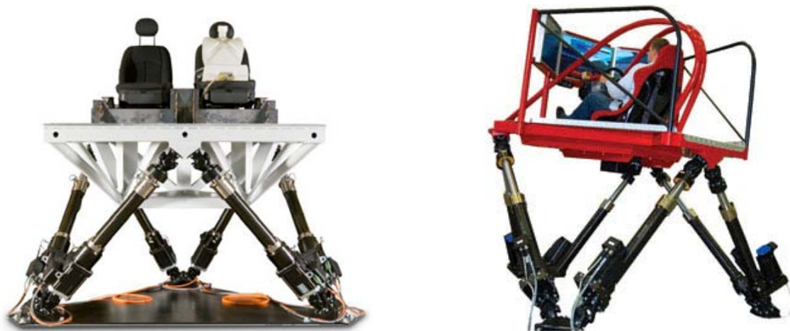
Left: ride-and-comfort shaker, right: driving simulator.
