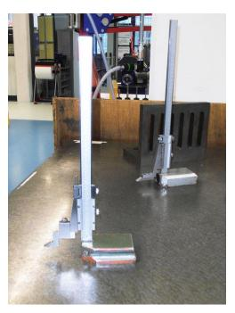
At the zero point, the scriber is flat on the surface plate with the scriber reading zero on the scale. Set the scriber to the desired height using the vernier graduation, and scribe a horizontal line on the material with the scriber. Then do the same for the vertical line (in which case the material needs to be turned 90°).
