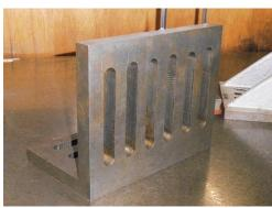
When marking off on the surface plate, a right-angled support may be used. This means sheet material, for example, can also be marked off on the surface plate.
