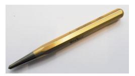
A small blow is given to the centre punch using a small hammer at the intersection of the two lines to create a small indent in the material. (The emphasis here is on 'small' to avoid buckling the sheet.) Centring is best done on a stable, non-springy base (e.g. a thick, flat piece of steel). This is where you want the drill to cut into the material. The small indent will prevent the rotating drill from wandering, and the hole will be drilled in the intended position.
