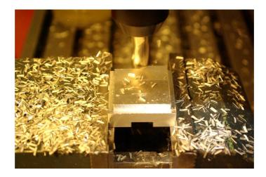
According to the diagram, four 6 mm keyways must now be made. Again, we take a cutter that is one size smaller and compensate for it, in both the width and length of the slot. The centre-to-centre distances of the slots are given, but with a smaller cutter another linear measure than the given centre-to-centre distance must be milled, to compensate for the smaller diameter of the cutter.
