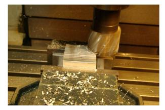
The method of plain milling and then milling the other side to thickness ensures that all sides have the same surface, rather than one side being clean and the other still having mill scale.
