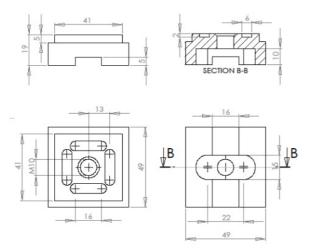
In this case, first the underside of the workpiece is machined, as shown in the bottom right of the diagram. We do this to cut both slots on the underside and part of the top side without having to change tools. The continuous slot of 16 mm wide and the keyway of 15 mm wide are both made with a 14 mm cutter.
