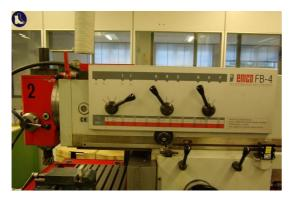
To machine the sides and the top of the workpiece, we use a side and face cutter in this case. We set the speed of the cutter using the gear levers on the side of the slide.
