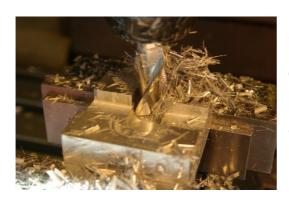
Subsequently, the keyway can be milled in the same way as the slot: first 5 mm deep (the maximum depth of one cutter pass), after which the cutter is set to the required depth in the hole while rotating and the keyway is milled at depth.
