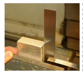
Once the rolled sides have been milled to size, the sawn sides can be made perpendicular to the milled sides. To do this, we use a try-square, with the stock part set on the supporting plates and the blade upwards. The supporting plates are parallel with the table. The plain milled side is pressed against the blade of the try-square. Once the sawn side has been milled flat, it will be perpendicular to the plain milled sides (in this case the workpiece must not be hammered on the bearing plates).
