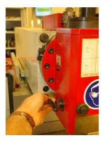
Before milling, a check is done to ensure that the quill clamp is secure. This clamp may only be loose during drilling, because otherwise there could be play in the cutter spindle during milling. This play may increase when the cutter hits the material, which can lead to the spindle having an impermissible play in the cutter head.
