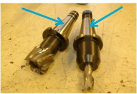
Initially, the cone and cone holder are clamped together in place. It is therefore important to keep the cone and the cone holder clean to prevent damage, which leads to imperfect clamping and off-centred turning of the cutter.
