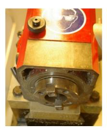
The cutter head cone is secured in the cone holder of the cutter holder in the direction of rotation by studs on the cutter head cone. The cutter holder has slots into which the studs fit. On top of the cutter holder there is a hole with an internal screw thread. To secure the cutter holder in the cone holder, this is tightened by an clamping shaft with a screw thread located in the cutter head spindle. This clamping shaft is moved using a square-head wrench.
