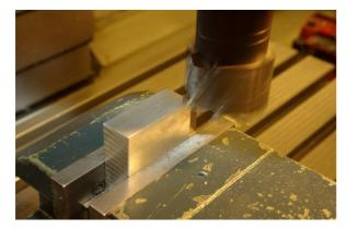
While the cutter is rotating, we just touch the surface of the workpiece. Now we know what zero is in the Z-direction and record this on the nonius or the digital readout. We move the cutter away from the workpiece and set it a few tenths of a millimetres lower. This side is now plain milled.
