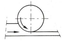
The resulting chip starts out thick and ends thin.
