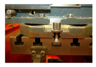
The machine clamp is secured in the X-direction by T-bolts with rings and nuts that are shoved into the T-slots. When tightening the nut on the T-bolt, the machine clamp is secured to the table.
