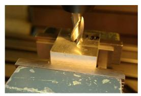
The middle is determined with the wiggler, and the zero point of the Z-axis is determined by the cutter by positioning it so it just touches the top of the workpiece. This is Z=0.
