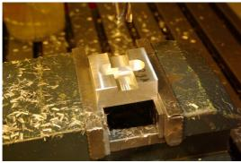
Now this side of the workpiece is finished, and the workpiece can be turned around.
