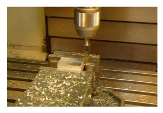
Because the diagram is measured from the middle, the middle of the workpiece must be determined. This is done using a wiggler, for both the X-axis and the Y-axis.
