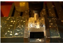
The smaller diameter of the cutter is compensated by positioning the cutter far enough from the centre line that it compensates the deviation of the radius from the planned radius. Thus, by positioning a 14 mm cutter 1 mm offcentre, both the + and – side of the 16 mm slot will be reached.
