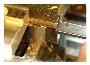
To avoid having to determine the centre again using the wiggler (reset and reposition tool), we first measure the distance between the side of the fixed jaw of the machine clamp and the workpiece. We do this using the depth spring of the slide gauge. This gives us a fixed point on the X-axis.
