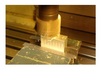
Once this is complete, we remove the workpiece and measure the height, and the excess material is milled off from the other side to achieve the desired dimension.
