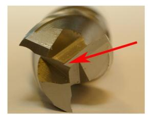
The universal cutter also cuts over the entire diameter of the face side as one of the cut edges extends over the centre line of the cutter.
