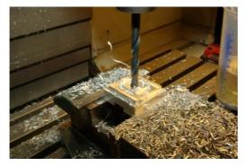
Depending on the drill bit to be used, a diameter for the centre drill bit is chosen that will drill 0.8× the diameter of the web of the subsequent drill bit.
